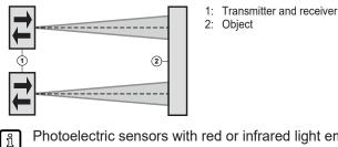
Photoelectric sensors with red or infrared light emit a cone-shaped light beam.
